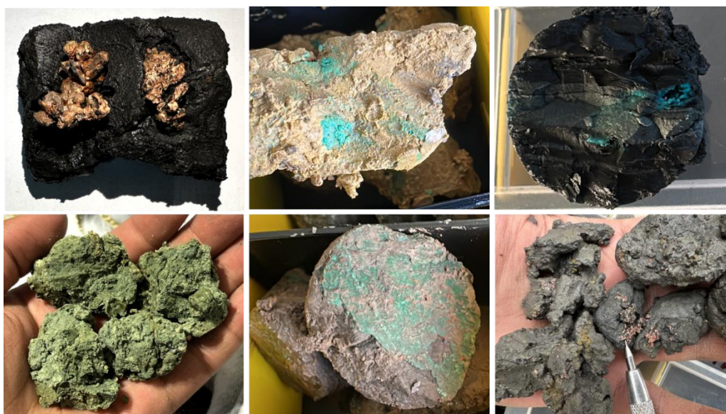
Figure 6: Copper oxides and native copper (malachite, chrysocolla, native copper) from drill samples.
