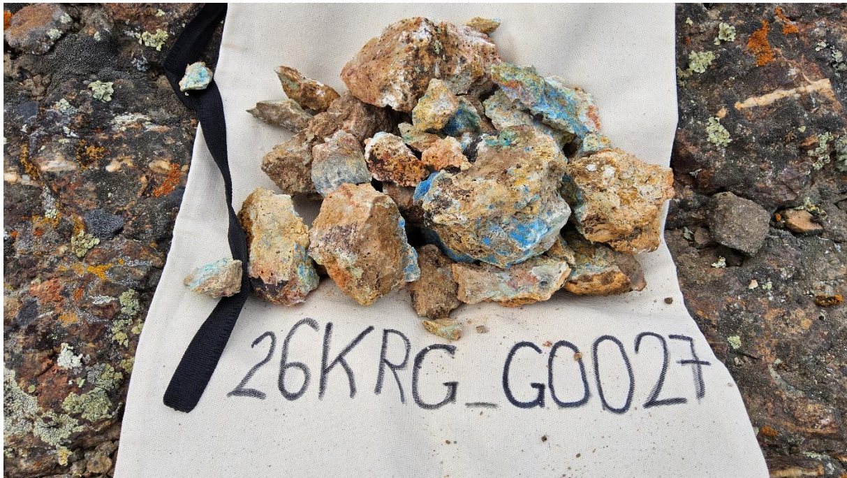
(Above) Malachite-azurite bearing samples from surface, (Below) Low sulfidation quartz veins prospective for gold mineralization.
